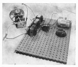
FIG. 5: The high voltage source can be used for effectively burning dust particles from capacitor plates.
