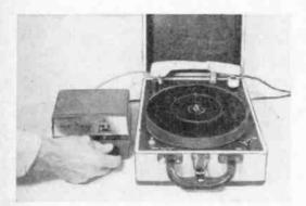
FIG. 1: A small FM tuner plugged into a portable record player gives dance music when the crowd tires of records. The wire bayely visible at left of tuner is a "built-in" antenna. FM plug cuts out crystal pickup and SPST switch idles turntable motor.
