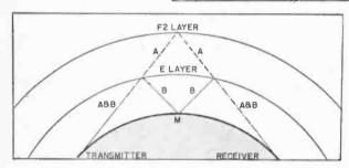
Fig. 3: This station is transmitting on two frequencies, A and B. A is the higher frequency which passes through the E-Layer where it is partially absorbed before being reflected back to Earth. Frequency B is reflected by the E-Layer and therefore suffers little in the way of absorption. It does suffer however, as it requires two hops. The strength of the received signals depends on what happens at point "M". SW Anyone?
