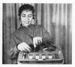
If unit fails to record, bridge terminals of record head with a pair of earphones to isolate the trouble. You should hear the program material.
