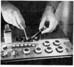
4 Clean heads periodically with commercial solvent such as Robins Industries head cleaner. Use soft cotton swab dampened with liquid. Do not drench.
