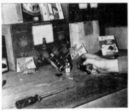
FIG. 5: Using thumb and gentle pressure, push out the rotor assembly. Do not hammer; push it carefully.
