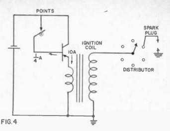
available voltage from the ignition coil diminishes. The voltage available from worn points is also a function of engine speed. Thus new points might make 30,000 volts available to the distributor for a wide range of engine speeds. But, after a considerable amount of use of this set of points, the available voltage will drop to something like 25,000 volts at 2000 rpm and about 15,000 volts at 4000 rpm.
