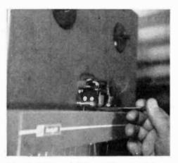
5 Use nail file with caution and you can fluff up a tired pressure pad. This treatment also takes oxide coat off pad surface. Do not scratch the heads.
