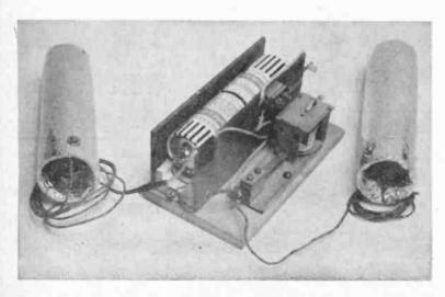
Fig. 1: Aluminum foil over the cardboard tube serves as the conductor. A surplus relay can easily be modified to serve as a vibrator to deliver the jolt where it's needed.
