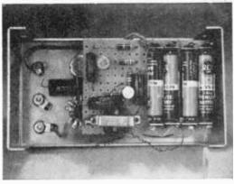
FIG. 6: Inside the box with the circuit board installed in place. Box and circuit board are wired separately, after installation, hooked up together.
