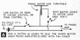
FIG. 6: Schematic shows location of SPST switch to idle motor when amplifier is used with FM tuner.
