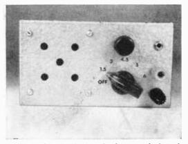
FIG. 5: Looking head-on at the front panel, the unit presents an uncluttered, business like appearance. Finish the panel with decal lettering and lacquer.
