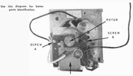
MOTOR COIL WITH LAMINATION
