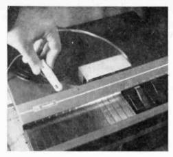
2 Stroboscope tape from Robins Industries appears to stand still when viewed under neon lamp provided speed is accurate. Speed changes also show.
