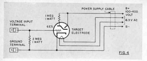
ring to the diagram will show the connections, and it may be used with any amateur transmitter that employs coaxial cable output. The power consumed by this indicator is in the microwatts, and negligible by any ordinary standards, so it does not waste valuable RF watts. It also indicates relative degree of modulation.
