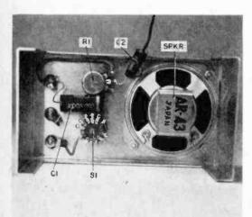
FIG. 4: Chassis-mounted parts inside the box cover include the speaker, switch, potentiometer, jacks and two capacitors. Wire these in place separately.
