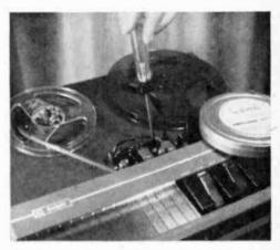
6 Align playback head by using Audiotex alignment tape. Carefully rotate adjusting screw until level reaches peak. Use non-magnetic driver.
