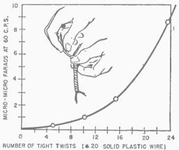
The chart shows the result of measurements made with a bridge at 60 cycles per
