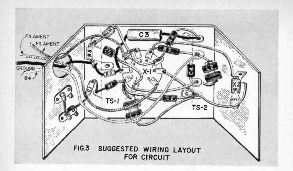
voltage. As soon as the plate voltage reaches 60-65 volts, the neon tube fires or glows, indicating the presence of an FM stereo signal.
