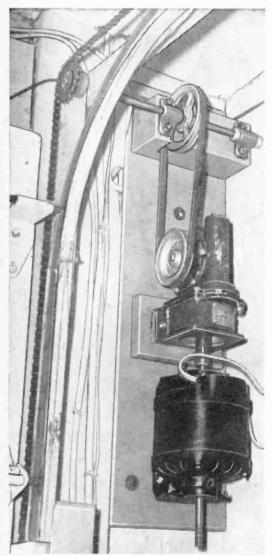
FIG. 1: The motor drive unit in a vertical mounted installation. A horizontally-based motor unit can usually be mounted easily in a vertical position.
