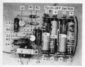
FIG. 1: Looking down on the circuit board, the parts are easily located. Wiring isn't critical, but try to keep leads as short and as neat as possible.
