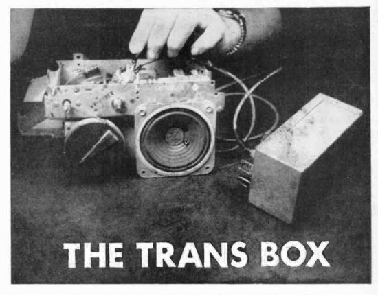
This compact two-transistor unit triples as an AF-RF signal tracer, utility amplifier, and transistor circuit power supply
