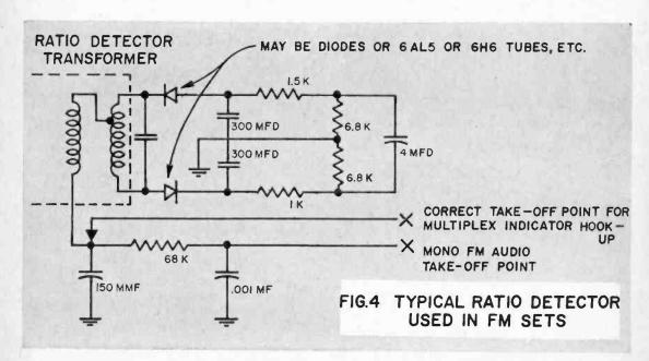
nected to J1 will be required. Use shielded cables in all cases. In this latter case the other end of the cable is connected to the output of the FM detector of your present receiver, ahead of any de-emphasis networks. Typical connection points for receivers using ratio detectors are shown in Fig. 4 whereas Fig. 5 indicates a typical hook-up where a discriminator type of detector is used.
