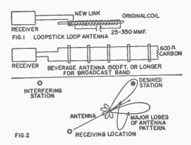
Resonate the original coil on the loopstick with a capacitor, to WQXR's frequency. Since WQXR is at the high end of the BC band, a small 50 mmf. miniature variable will do. When the loopstick is in the horizontal position it should show a null when it is rotated. Turn it so that the Paducah station is nulled out but WQXR still comes in. When you have found the proper position, you can fix the loopstick in place.
