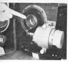
Fig. 12: Here's how the lens of the surplus TV camera is focused by the selsyn. Note rack and pinion set-up.
