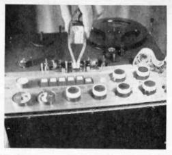
Use a demagnetizer such as this one from Audio Devices to remove unwanted residual magnetism from tape heads. Tape on pole pieces saves heads.
