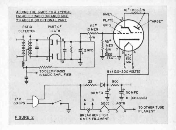
It can usually be found at the B-plus side of the output transformer, or at the rectifier cathode. A 1 megohm, ½ watt resistor (R1) must always be wired between the plate and target of the 6ME5.
