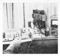
If you have a VTVM, you can connect a 100 ohm resistor in the ground leg and measure the voltage drop between the head and record amplifier.
