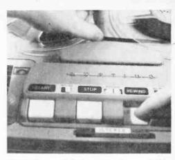
10 Unless you have tape lifters, by-pass the slot during rapid wind and rewind to save wear and tear on your head surfaces. Trip end-of-tape lever.
