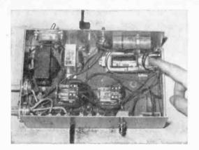
FIG. 8: The control box should be mounted on the wall near the motor drive. Location is not critical.
