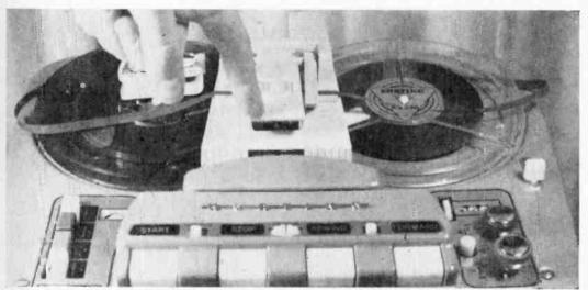
Fig. 10: Cut! The splicer cuts a 45° diagonal, in both pieces of tape. Apply the splicing tape over the cut, move the cutter head to trim, and press again. Result is "waist" cut, hence name "Gibson Girl."
