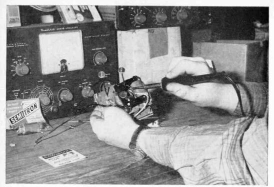
FIG. 1: Start the replacement by first disconnecting the wires from the clock motor coil soldering terminals.
