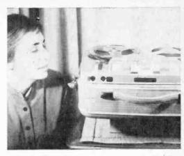
Fig. 13: Check for reel-warpage at eye level while reel turns. Any warp will quickly become obvious, reel eliminated before it could damage tape.
