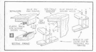
The edges of this cabinet were trimmed by ripping the angular edging from a length of ¾-in. x 8-ft. oak to the same thickness as the Masonite Royalcote. This was done on a table saw. However, you will save a good deal of time and effort by buying your edging ready-cut. Apply it with glue and hold it in place with clamps; then sand it. Miter the two top front corners and butt the front vertical sections against the joint.
