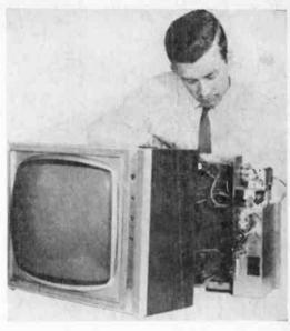
—Too bad there's not more about technical design of the Custom 70. Transformer power supply, bonded pic tube, 3 stages of video I.F., new high-gain tuner and one full year guarantee are features hard to find in commercially manufactured sets priced under \$200. Anyhow, that's our opinion.
