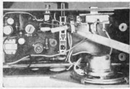
Fig. 2: The modified unit contains a simple push-to-make switch. Glue a tab to old switch to activate both.
