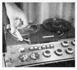
3 For more stringent test, splice sections of the strobe tape into beginning, middle and end of a reel, so you can test speed under full-load conditions.
