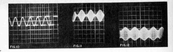
In cases where higher frequency is to be determined, a signal generator (audio or RF) should be used as the references source. The sweep selector switch is set to Hor. Input and the generator is connected to horizontal input terminals.
