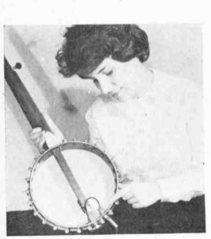
Fig. 1: Rubber-covered pickup is mounted on underside of head, beneath bridge. Cardboard shims hold in place.
