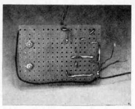
FIG. 2: Wiring is brought through the holes to the underside of the circuit board. Note that no components mount underneath for ease of servicing.
