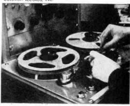
CUTTING the goofs is the tricky job of the tape editor. Ease in cutting, splicing is advantage of tape.
