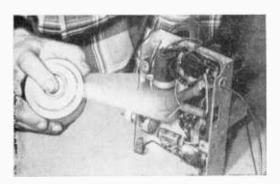
haves or goes dead. The trouble may be a part that expands with heat after current has been flowing through for a few moments. Spray suspicious parts with CO2 gas one at a time. The intense cold will contract a defective component so it can work normally.
