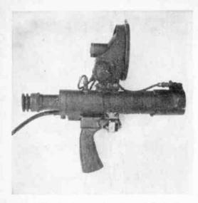
FIG. 3: Famed sniperscope is now an excellent police weapon with its built-in, infrared searchlight. A well adjusted scope can "see" up to 300 ft., but it still isn't up to the Army's new night vision equipment.
