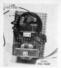
Fig. 3: Using the schematic (Fig. 4) and the photo above, build the unit on a small piece of perforated phenolic.
