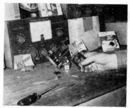
FIG. 4: Removal of the screws "A" and "B" permit the motor coil and rotor to be disassembled from the frame.
