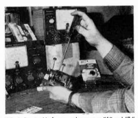
FIG. 7: Reassemble frame, replace screws "A" and "B."
