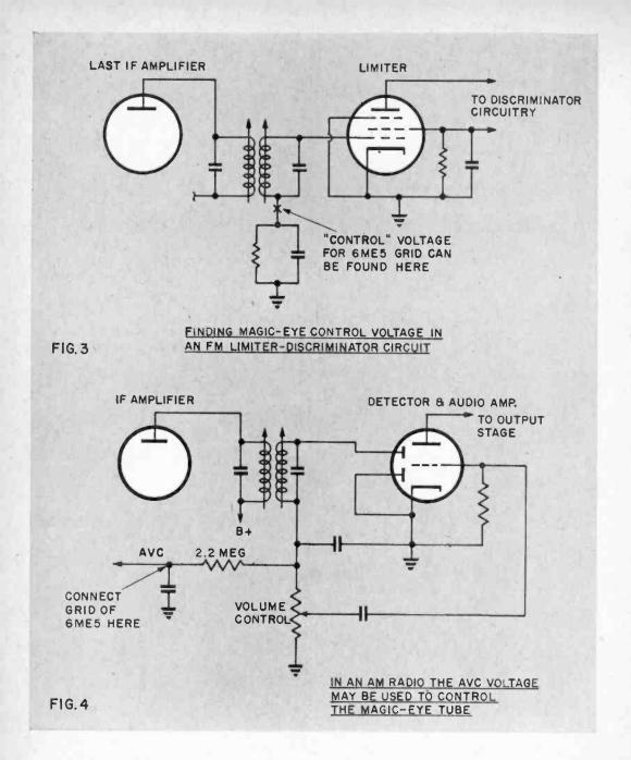
rating, it may be used in series with the existing tube filaments. In the Granco, it was most convenient to break the series-string at its beginning (pin 4 of the 50C5). Since the 6ME5 filament (pins 3 and 4) is isolated from the cathode, it is not necessary for either side of the filament to be grounded, and it may be placed in the series-string at any convenient point. Although the voltage
