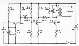
2. SCHEMATIC for transistor amplifier which boosts sound.
