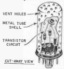
you have a plug-in device that fits tube sockets. If components such as resistors radiate heat, then drill enough vent holes to provide an adequate air circulation.—John A. Comstock.
