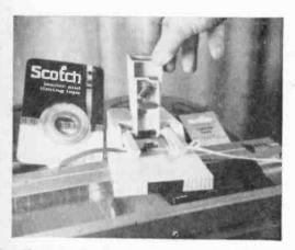
Fig. 5: Leader tape, an uncoated polyester saves end wear when threading, prevents valuable taped information from being lost. Also used for timing.
