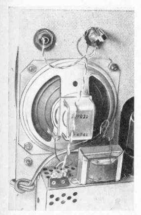
FIG. 2: Closed-circuit jack is wired into pickup leads and is mounted as close as possible to the pickup.
